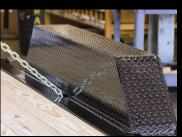
Tie Down Between Fenders (flush w/deck & fenders)
