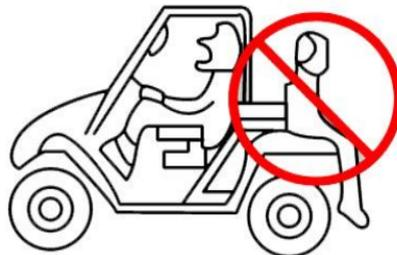
The total weight of operator, passenger, accessories, cargo, trailer tongue weight, and the vehicle itself must not exceed 845kg (1861lb). Carrying a passenger and cargo can affect vehicle handling.
