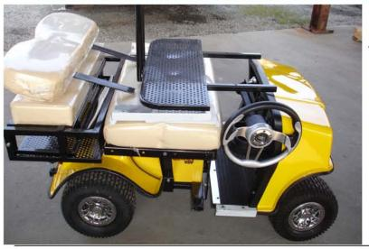
First, remove the rear step plate, the front seat back, and the protective barrier\* on the front seat. Put these items aside (out of your way) until you're read to install them.
