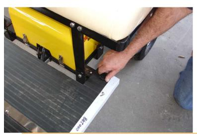
g. Finally, replace and tighten both left and right locking knob bolts to secure floorboard extension securely to vehicle chassis.
