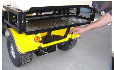
b. Insert both step plate bars into rear chassis frame tubing and gently guide both bars all the way in, until secured firmly. (Use step plate safety bar to help complete this installation procedure.) Then just hand-tighten both locking nuts.
