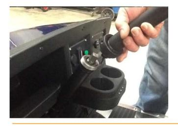
b. To reinstall make sure steering wheel is straight for driving because it will fit in four different positions, line up square steering shaft with square tube and screw large nut on until it is finger tight.
