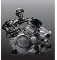
62 HP, liquid cooled, twin cylinder, 8-valve featuring Delphi® Electronic Fuel Injection and CVTech clutching.
