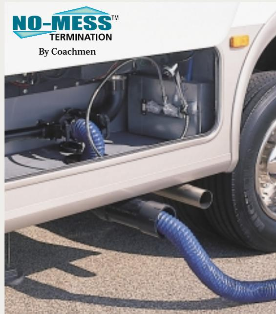
The Coachmen exclusive **No-Mess™ termination system** is an easy to swivel boom arm that provides a convenient storage location for the termination hose. Your storage bay stays cleaner and the hose can remain connected after use.
