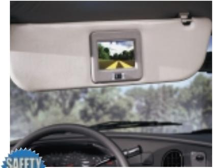
**SAFETY FIRST** The optional rear view camera provides you with peace of mind and confidence as you back up. It is cleverly designed into the sun visor so that it takes up minimum space, yet it is large enough to give you a solid rear view.
