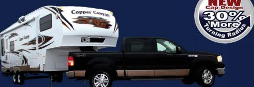
Sprinter's new cap design allows short bed trucks with extended cabs to turn an additional 30% without making contact with the front cap.
